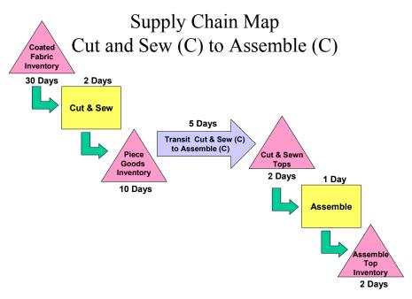
Figure 4. Supply Chain Map Cut & Sew to Assemble
